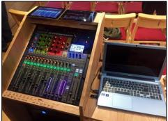
The bespoke console houses the Soundcraft Si Expression digital mixer with wireless iPAD control for operation anywhere within the Church. The system provides over 70 audio inputs and outputs for maximum flexibility and system growth potential.
